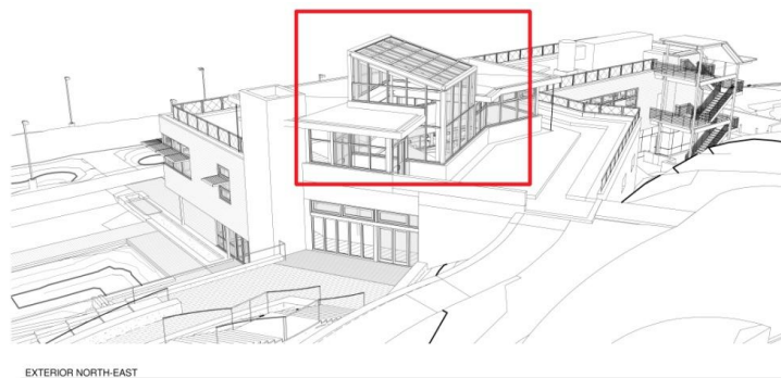
Figure 6 - View of exterior from northeast site. Lantern outlined in red.
